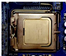
Fig. 4 Once the CPU is properly inserted, please replace the load plate and push the metal lever back into its original position.
